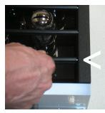
To complete the installation, press the bar in the direction of the pin already inserted, and manoeuver the other end into the corresponding dimple in the other side rail, then release.
