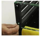
Insert and tighten the remaining three screw/cone washer assemblies.
