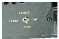
The illumination of the front VAC logos may be dimmed or turned off via a switch on the back panel of the power supply.
