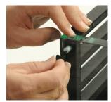
Insert one of the provided screw/cone washer assemblies into one of the top holes in the glass. Start the screw, taking care that the threads align properly. Tighten as much as you can using only your fingers.
