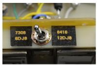
Units from serial number 1009901 can use either type, but you MUST set the tube type switch correctly.
