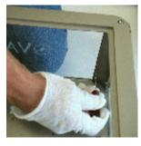
Tighten the four white nylon setscrews that secure the front glass using the tool provided. Turn clockwise to tighten.
