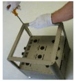
Replace the four screws that secure the top frame. Turn clockwise to tighten.
