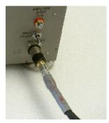
In many systems a lower noise floor is achieved with RCA single-ended sources by using the lower RCA jack adjacent to the XLR input.
