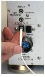
04) For traditional stand alone operation, set the 12 volt trigger switch to "manual". To use a 12 volt trigger to control power on/power off, set the switch to "automatic". Also select "automatic" when connecting to the iVAC data buss of the Phi 2.0 Master Control Preamplifier.
