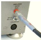
RCA (single ended) connection normally is made to the RCA jack on the rear panel. This is the "direct in" mode.
