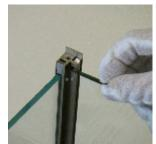
Tighten the metal setscrews that secure each block using the allen key supplied. Turn clockwise to tighten.
