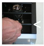
To complete the installation, press the bar in the direction of the pin already inserted, and manoeuver the other end into the corresponding dimple in the other side rail, then release.
