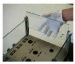
Slide the side glass plates into the pillars' channels.
