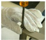
Wear the supplied cotton gloves to minimize the chance of fingerprinting the nickel plated chassis. Wipe any oils off immediately.
