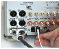
Connect the iVAC data communications cable to an associated Phi Power Amplifier if appropriate. This allows the preamplifier to control power on, power off, and logo illumination intensity.
