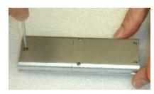
To install or change batteries, first loosen the screw on the back of the remote.
