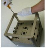
Remove the four screws that secure the aluminum top frame to the chassis pillars using the tool provided. Turn counterclockwise to remove.
